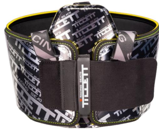
Maximum front adjustment is achieved when there is a minimum of 10 mm of Velcro overlap between the main front strap and the front hook velcro receptor.
